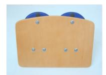
necessary to be tight. The imbedded "T" nuts could be forced out of the pod, so save yourself a problem and only snug-up.
