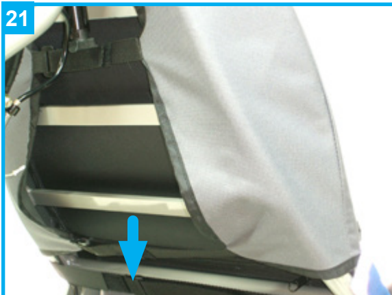
21. Unloop Velcro Strap through the D-ring, underneath the foot well.
