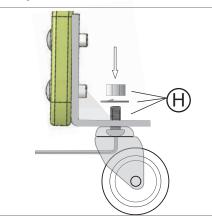
Install brake casters in the rear for stability. Use allen key to insert bolt up through the caster and bracket. Tighten nylon nuts with a crescent wrench. Note: Maintain tight screws.
