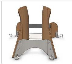
Attach (D) front brackets to (A) wooden sides with (4x) bolts. Finger tighten bolts first, then securely tighten with wrench. (Important : attach bracket to inside as shown)
