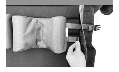
25. Lift Base Fabric Legrest Section and wrap Calf Cushion Attachment Straps around Base Fabric Legrest Section and through opposite Strap Guide Holes as shown here.
